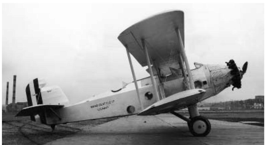
**A TG-1, a Great Lakes-built T4M-1, with its underslung torpedo. T4Ms and TGs had a relatively long career in the Navy from 1927 to 1937.**
