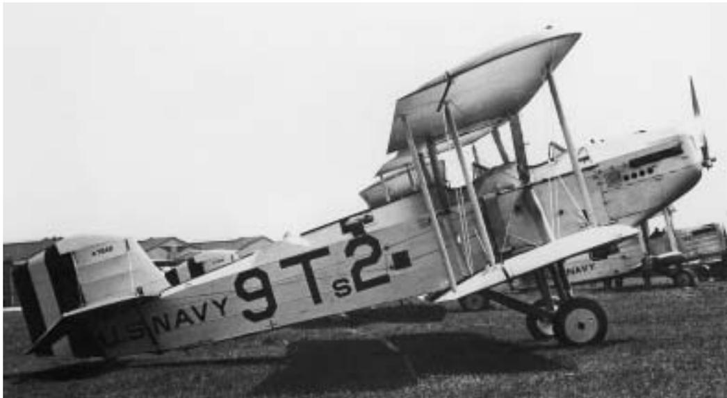
**The Martin T3M-2 gave the Navy the capability to operate torpedo planes from carriers.**
