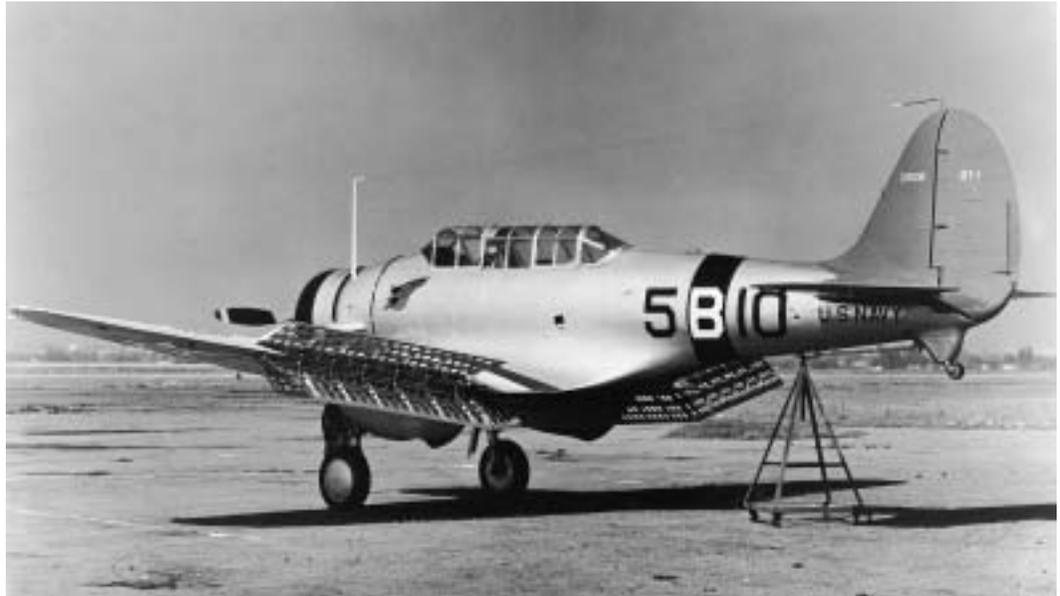
The BT-1's landing gear retracted aft into external housings under the wings. This is the XBT-2, a BT-1 modified with fully retractable landing gear.
