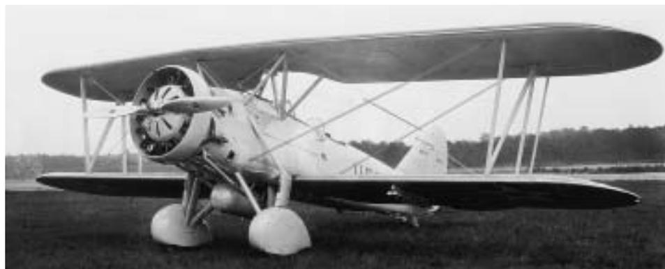
The Martin T5M was approved for Navy service and given the designation BM-1 in the new bomber series. Note the sling beneath the nose of this BM-1 to make sure the bomb clears the prop when released in a dive.
